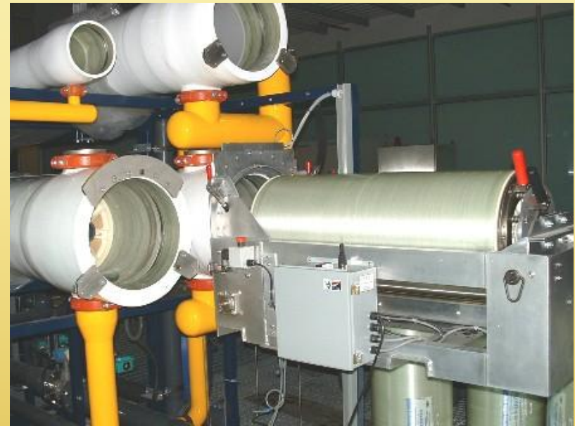
Loading tool attached to 16-inch pressure vessel
